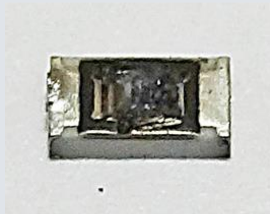
V司抗浪涌 1206 CHIP型电阻 (100Ω、5%)
