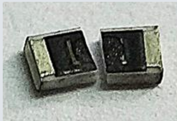
Y司抗浪涌 1206 CHIP型电阻 (100Ω、5%)
